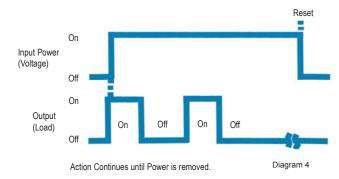
Upon application of input voltage, the relay contacts transfer and a preset delay begins. At the end of the preset delay, the relay contacts drop out and remain in that condition for a second, independently adjustable preset time. At the end of this time, the relay contacts pull in and the sequence repeats until input voltage is removed.
